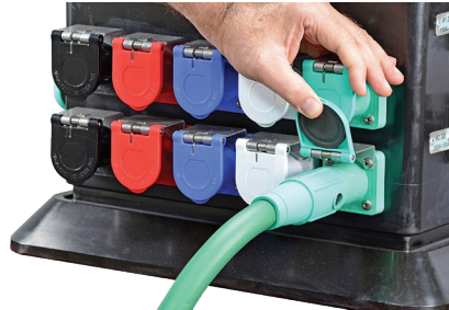
Insert the Cam connector into the receptacle and rotate Cam connector at least 90 clockwise degrees to lock
