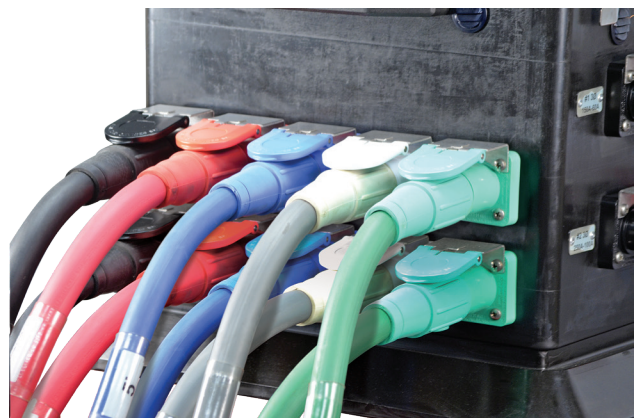
Insert the Cam connector into the receptacle and rotate Cam connector at least 90 clockwise degrees to lock
