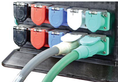
Insert the Cam connector into the receptacle and rotate Cam connector at least 90 clockwise degrees to lock
