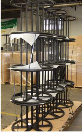
Lex was able to improve the cable reels specified by the Marine Corps by making them stackable.
